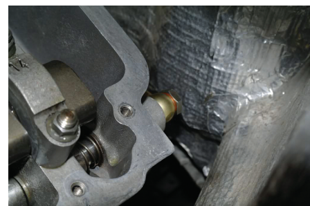
Additional oilfeeds to increase oil flow and assist cooling on the exhaust side of the engine
